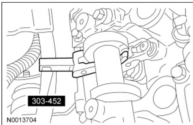
5. Use compressed air in the cylinder to hold the valves in position.
