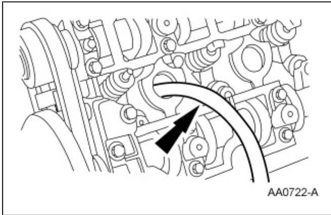
6. Install the Valve Spring Compressor Spacer between the valve spring coils to protect the valve seal from damage.
